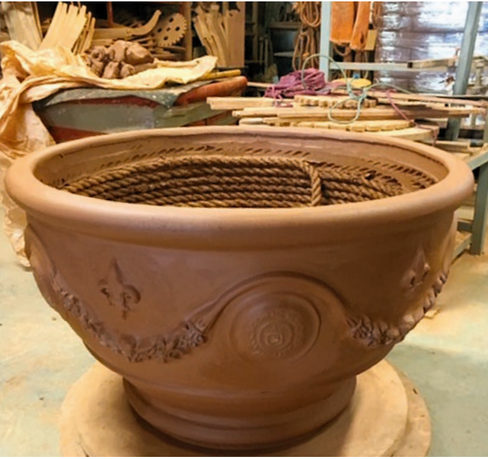
An Anduze cup being prepared in Fourbet's workshop in France; it can take a week to slowly remove all the rope.
