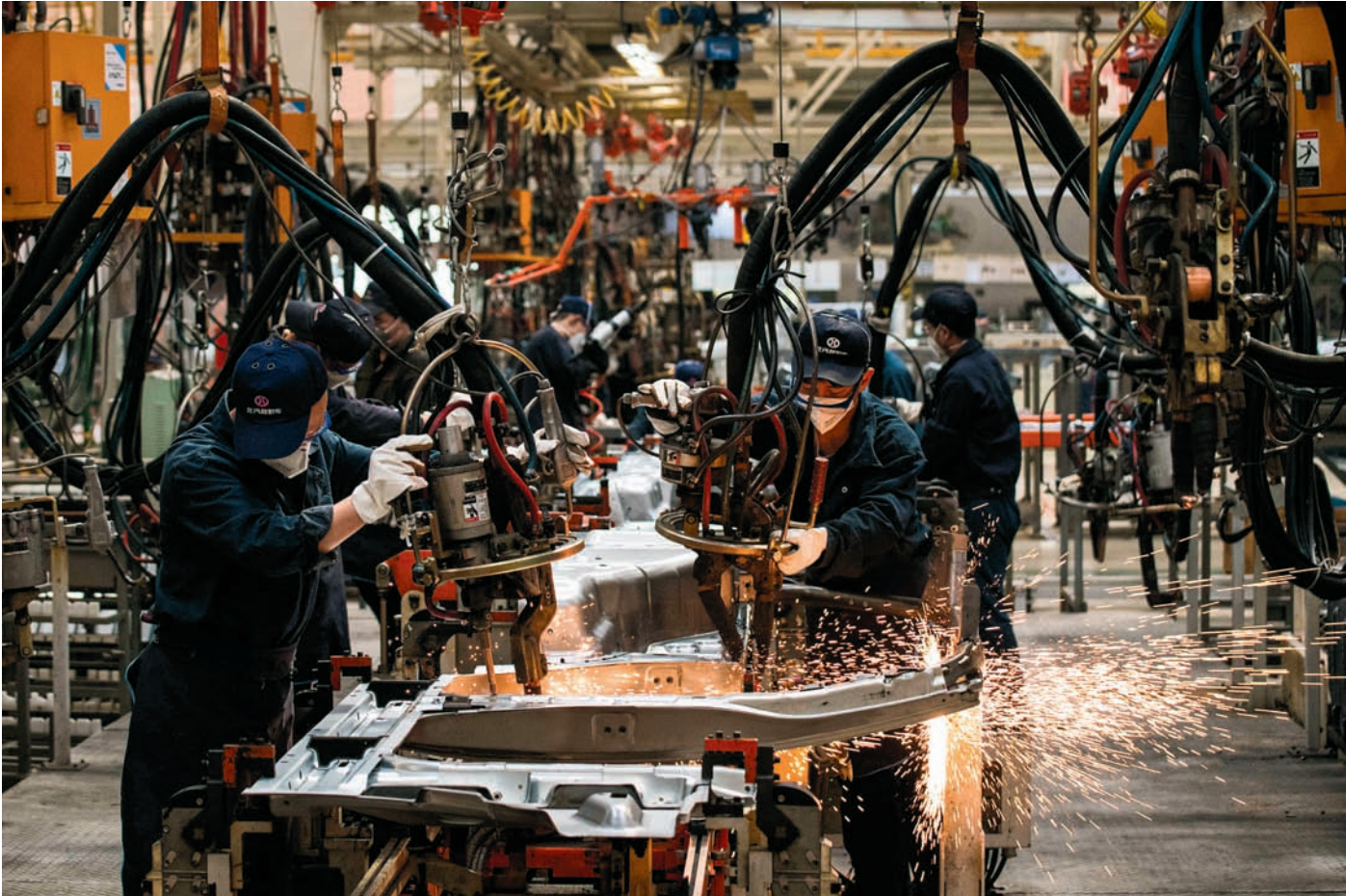
Workers at the Beijing Automotive Group weld SUV parts on an assembly line in Beijing on Aug. 29, 2018.
